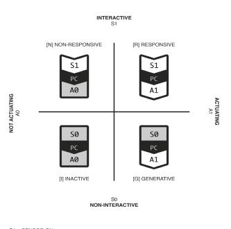
\$1 = SENSOR ON \$0 = SENSOR OFF A1 = ACTUATORS GENERATE OUTPUT A0 = ACTUATORS DO NOT GENERATE OUTPUT
